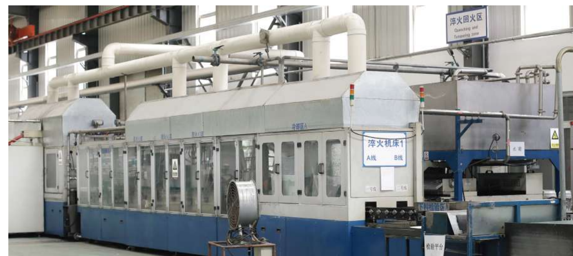
Fully automatic high frequency induction quenching/straightening production line for side door impact beam
